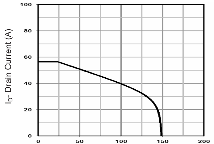
T_J -Junction Temperature (°C) Figure 9 Current De-rating
