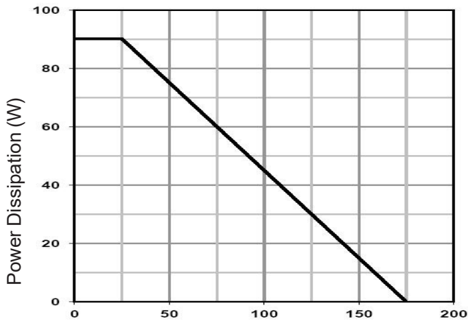
T_J -Junction Temperature(°C) Figure 7 Power De-rating
