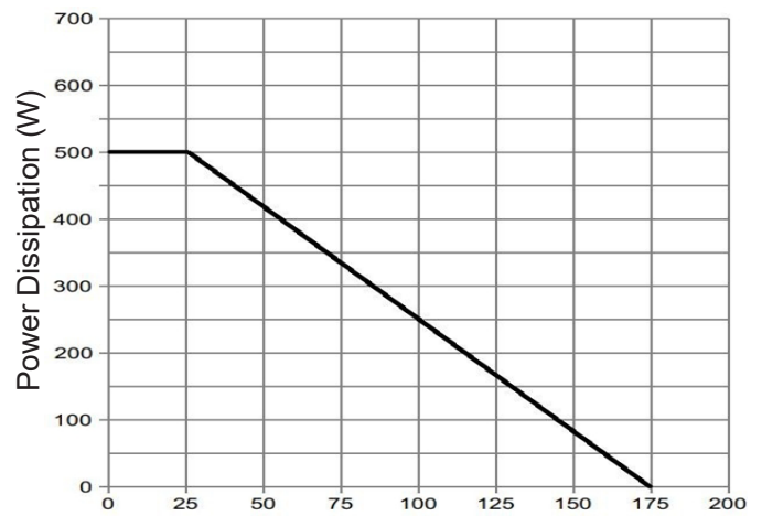
TA-Case Temperature(°C) Figure 9 Power De-rating
