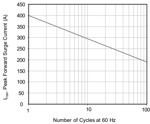
Figure 7 - Maximum Non-Repetitive Peak Forward Surge Current
