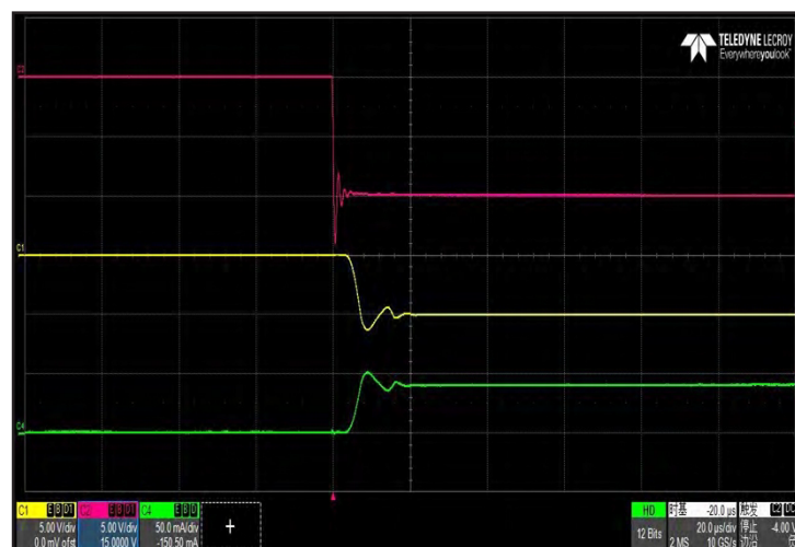
VS79L05E, V_{IN} = 0 \sim -10V , I_{OUT} = 40mA
