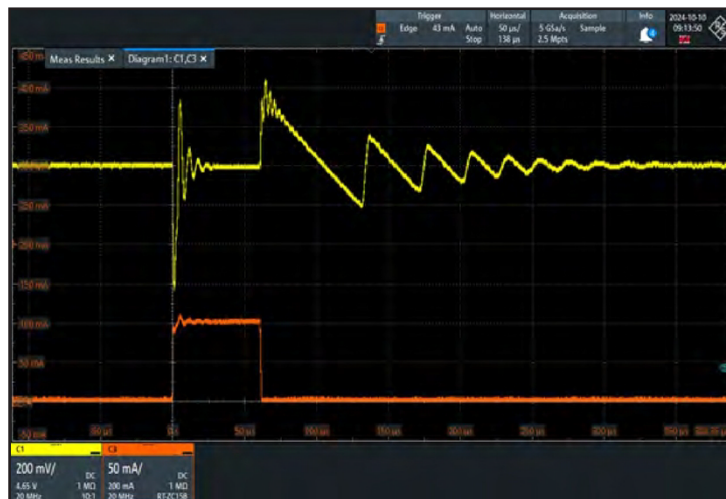
VS79L05E, V_{IN} = -10V , I_{OUT} = 0mA \sim 100mA
